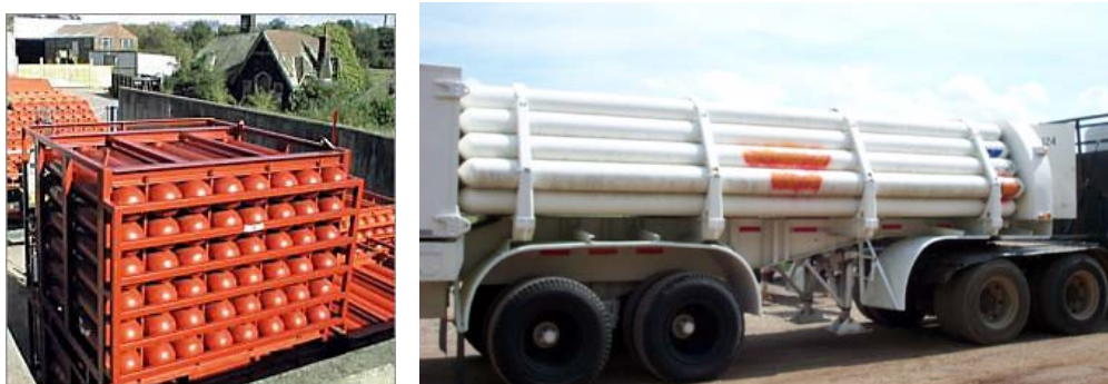
Fig. 2-19: CGH2 Cylinders [source: Air Products] and tube trailer [source: http://www.fibatech.com ]
