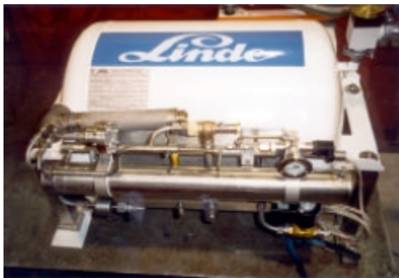
Figure 2-24: example of on-board liquid hydrogen tank [source: Linde AG]
