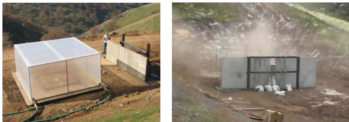
Fig.5-21: Experiment of hydrogen explosion and RC structure damage (left:Experimental system, right:A moment of explosion)
