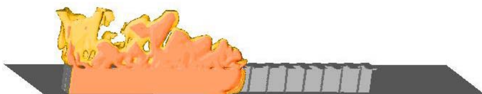
Figure 5-16 Computational Fluid Dynamics can be useful when estimating required venting. Distributed venting, like the transverse venting shown above [Hansen, 2005], can be very efficient to keep pressures low. CFD-tools can take into account detailed layout, including shape of vessel, position and shape of vent openings, presence of geometry and more. In addition to maximum pressure, shape and duration of pressure as well as distribution in space can be found using CFD.
