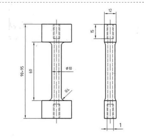
Tensile specimen for hydrogen tests (hollow tensile specimen) (can also be performed with specimens cathodically charged or with tensile spencimens in a high pressure cell)
