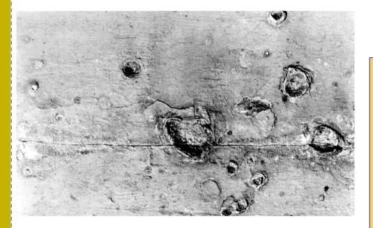
FAILURE OF A HYDROGEN TRANSPORT VESSEL IN 1983. HYDROGEN CRACK INITIATED ON INTERNAL CORROSION PITS
