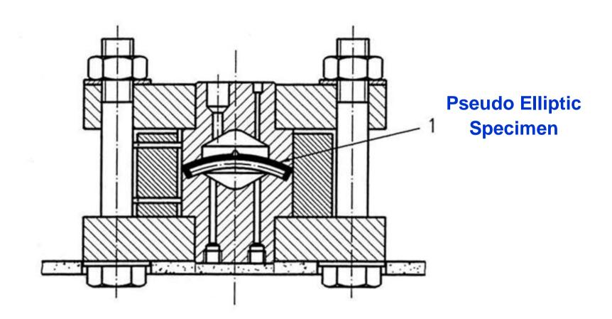
Cell for delayed rupture test with Pseudo Elliptic Specimen
