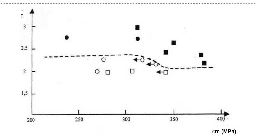
Hydrogen embrittlement indexes (I) of reference materials versus maximum wall stresses (σm) of the corresponding pressure vessels
