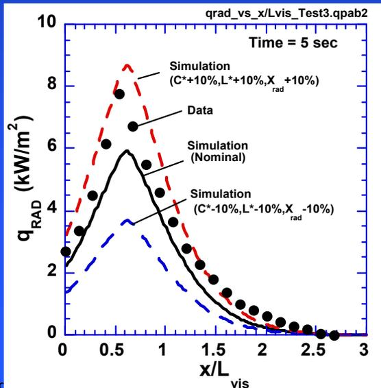
Comparison of Simulations with Heat Flux Data
