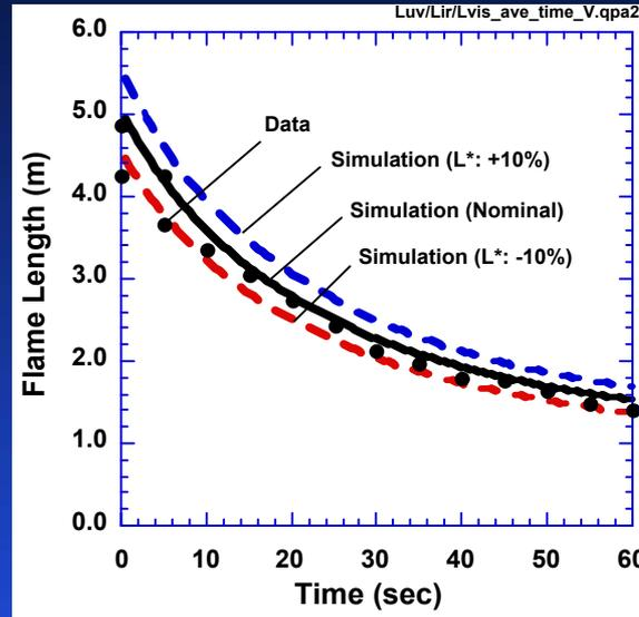
Simulation of SRI/Sandia Jet Flame Experiment
