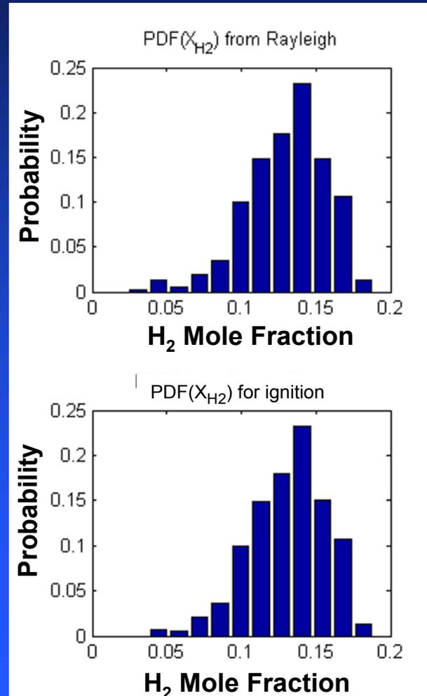
⇒ Unconditional PDF's of H<sub>2</sub> concentration near centerline show wide range of H<sub>2</sub>/air mixtures but no pure air.
