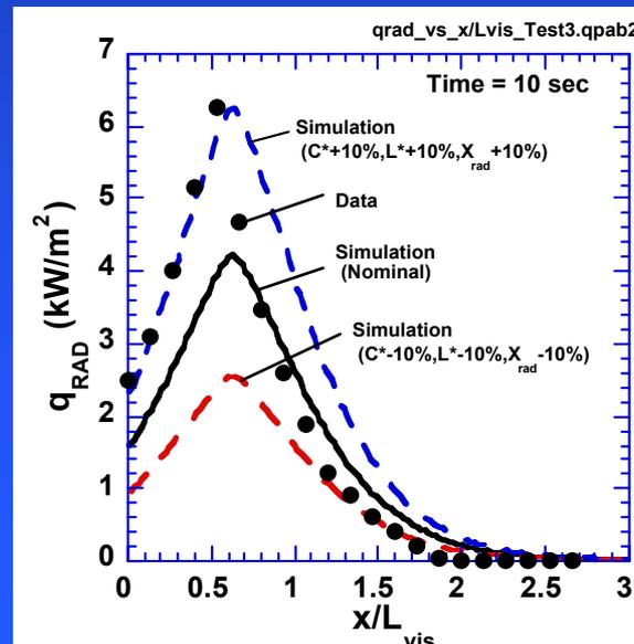
Comparison of Simulations with Heat Flux Data
