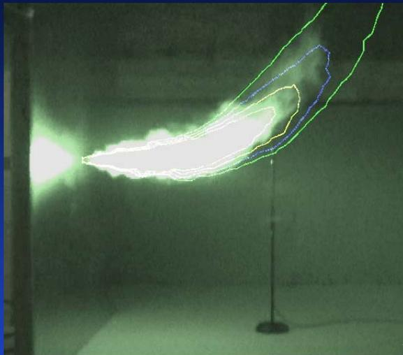
Jet Flame from an Ignited H<sub>2</sub> Slow Leak\*
