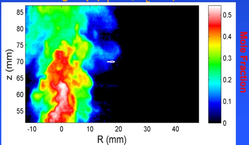
⇒ In the lower image both local ignition and jet lightup occurred since mixed  $H_2$ /air was present at the ignition point and within the flammability limits.
