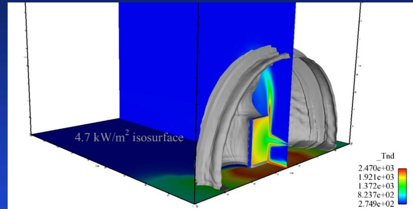
Free jet flame radiation heat flux comparison with experiment
