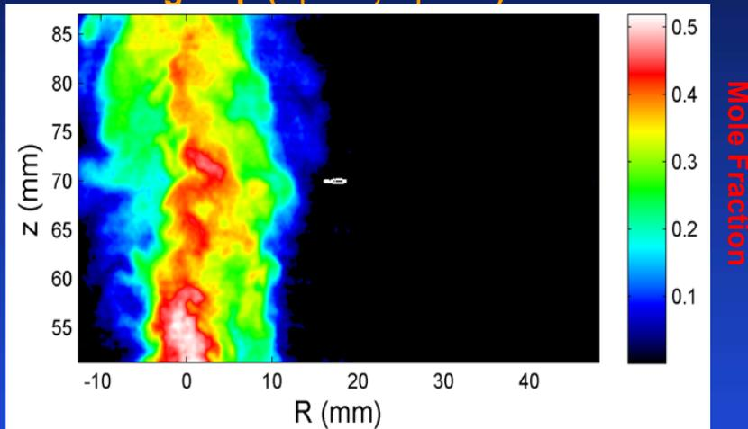
⇒ Instantaneous concentration distribution near ignition point at radial location in outer jet shear layer.
