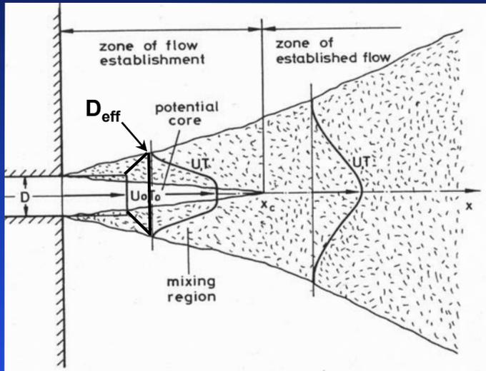
Effective diameter nozzle expansion for underexpanded jet
