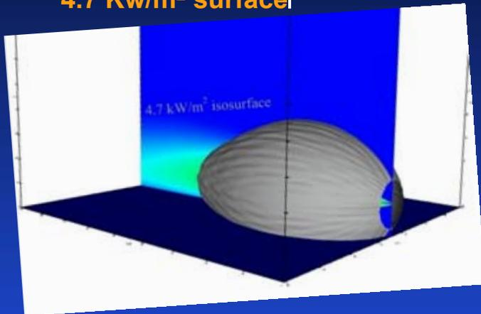
H<sub>2</sub> Jet Flame Impinging on Barrier
