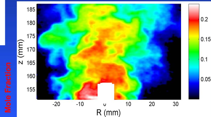
Use simultaneous Rayleigh imaging and laser ignition to characterize H<sub>2</sub> concentration distribution at ignition point.
