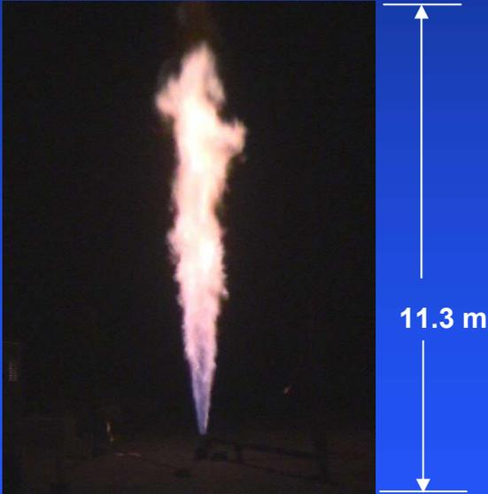
**Nighttime Photo of H<sub>2</sub> Jet Flame Test**
