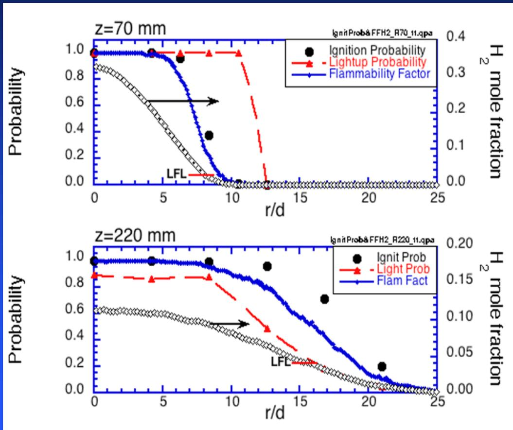
Ignition measurements based on 100 mJ spark at 3 sec intervals.
