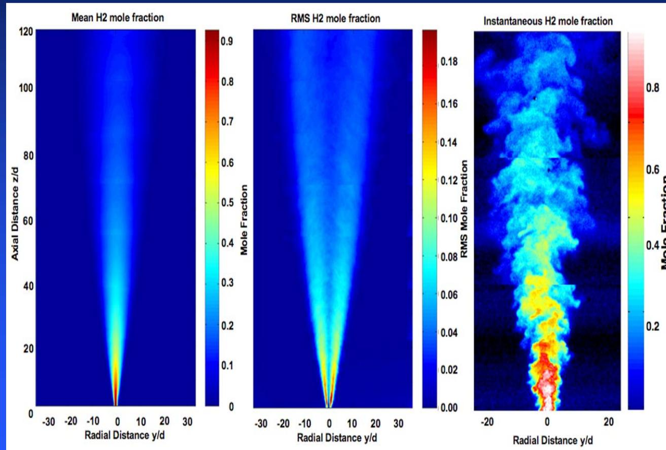
⇒ Time-averaged mean and fluctuating concentration field provides validation data and link to CFD modeled quantities.
