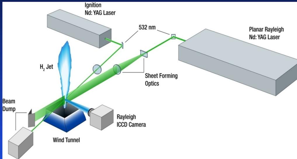
Rayleigh laser occurs 320  $\mu\text{sec}$  before ignition laser pulse.
