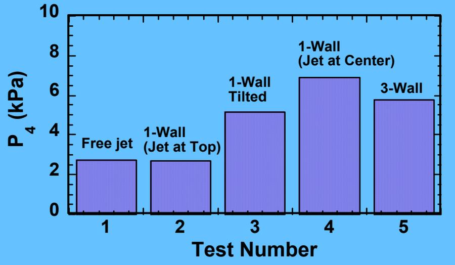
⇒ Wall-centered jet results in a factor of 2.5 increase in overpressure prior to wall.
