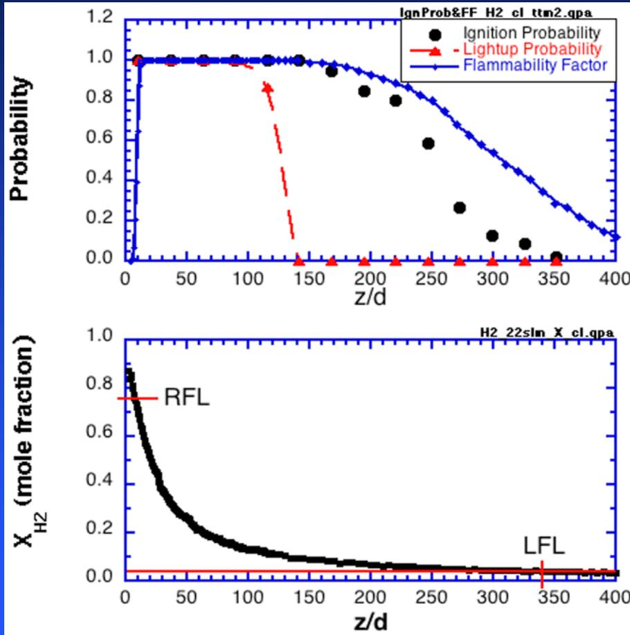
Ignition measurements based on 100 mJ spark at 3 sec intervals.
