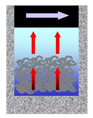
Heat removed by evaporation Heat dissipated through cover water
